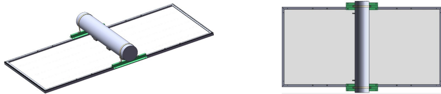
Installation of a module with the single-axis tracking system
